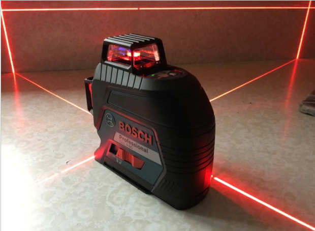
13. Floor levels checked with laser level
