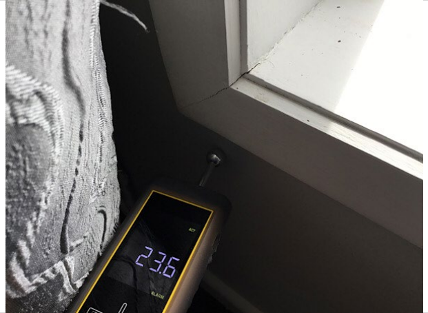
14. Typical low moisture reading below windows
